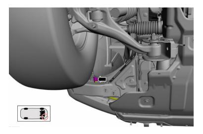
7. If equipped, remove the bolts and front bumper bar using a T40 socket.
