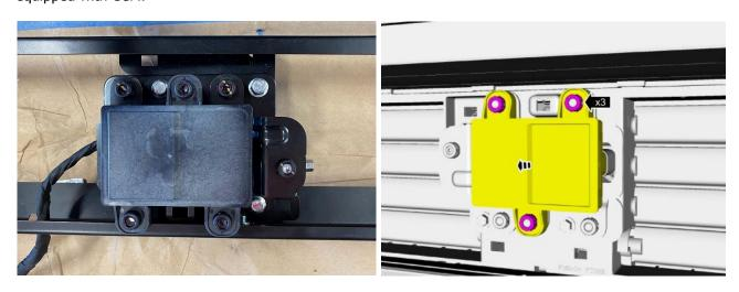
20. Remove the active grille shutter motor from assembly by remove U-shape brace, then removing shutter arms from motor. Install on new supplied bracket using the (2) supplied zip-ties.
