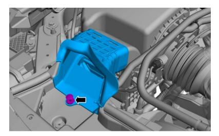
31. Remove the 4 bolts securing airbox lid to airbox. Remove stock filter by lifting up and away.
