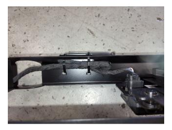
22. Install the new CCM bracket assembly to vehicle using the (4) factory fasteners. Torque to 62 in-lb using 8mm socket.
