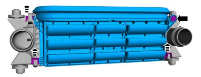
18. Set CAC to stock brackets. With the aid of a 2<sup>nd</sup> person, install the (4) bolts from the IC/tow hook brackets to install CAC. Torque to 59 ft-lb.
