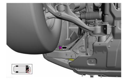
29. Reinstall the fasteners and the engine front under shield. Torque to 124 in-lbs.
