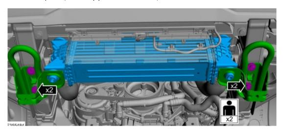
16. Remove the CAC isolators from CAC. Transfer to new CAC.
