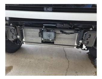
23. Reconnect CCM wiring connector to CCM. Reinstall plastic cover over CCM bracket, this will **NOT** fit after bumper installation.
