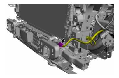
12. Remove the (4) bolts and the lower active grille shutter unit using 8mm socket.
