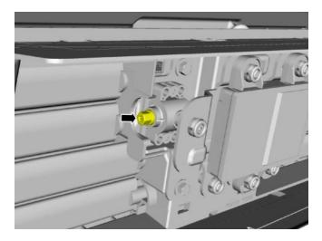
36. **NOTE:** Measurement must be taken from the non-raised side of the CCM. Place a combination square level on the face of the CCM and check the alignment.
