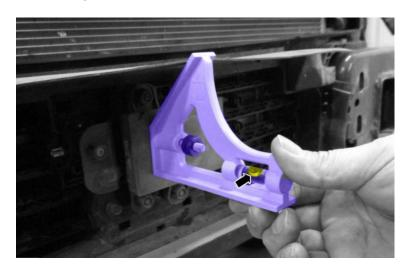
37. **NOTE:** Measurement must be taken from the non-raised side of the CCM. Keeping the combination square level on the face of the CCM, adjust the pitch by turning the adjustment screw until the CCM is vertical and level.
