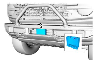
11. Disconnect the lower active grill shutter actuator electrical connector.
