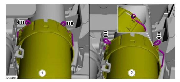
5. Release the CAC outlet pipe by spreading the retainer ends outward. Position the retainer ends in the notches locking the retainer in the open position and position aside the CAC outlet pipe.
